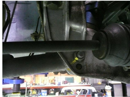
Front control arm pivot raised 20mm
