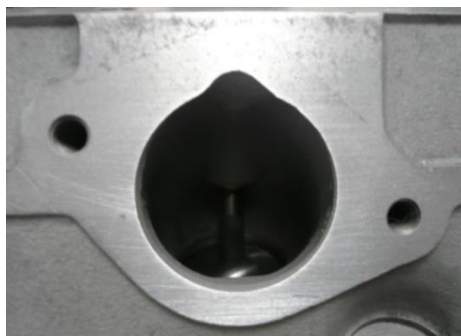
Intake port – Typical diameter 40.8mm
