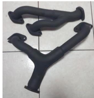
Porsche 944 Fabricated exhaust manifolds
