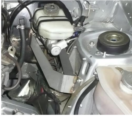
Example of brake master cylinder brace
