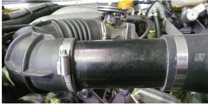
70mm diameter tube that replaces mass air flow meter
