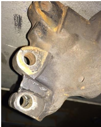
Typical strengthening gusset welded to stub axle.
