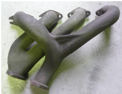
Porsche 944 Cast exhaust manifolds
